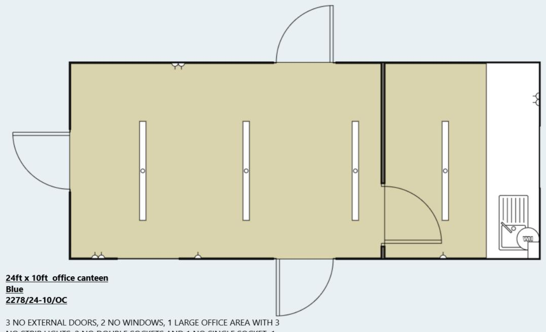
3 NO EXTERNAL DOORS, 2 NO WINDOWS, 1 LARGE OFFICE AREA WITH 3 NO STRIP LIGHTS, 2 NO DOUBLE SOCKETS AND 1 NO SINGLE SOCKET. 1 NO INTERNAL DOOR LEADING TO KITCHEN AREA WITH 1 NO STRIP LIGHT, 1 NO WORKTOP, 1 NO SINK, 1 NO WATER HEATER, 1 NO ELEC BOX, 1 NO DOUBLE SOCKET & 1 NO SINGLE SOCKET
